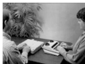
The sighted partner uses the TDD by typing on a typewriter keyboard and seeing the messages on a visual display. The deaf-blind partner keys in messages on the braille keyboard and reads messages on the braille display.
