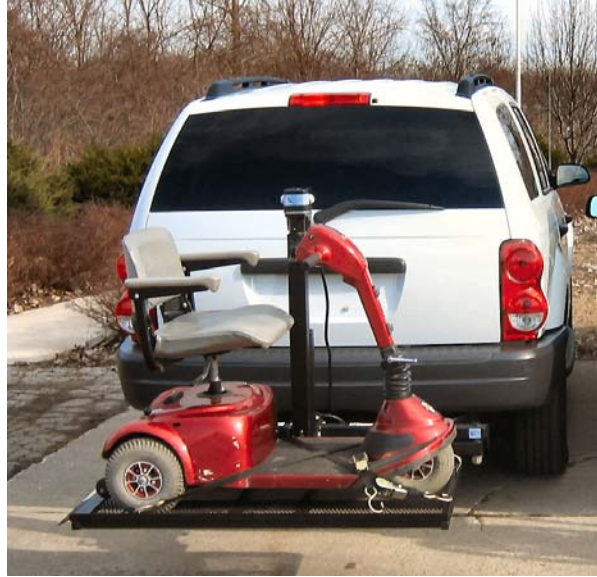
Figure 4: The Lift 'N' Go Model 210 electric powered carrier from WheelChair Carrier is mounted on the hitch of a car, truck or van.
