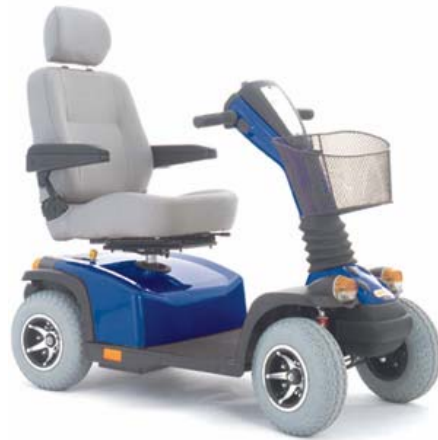
Figure 2: The Legend XL from Pride Mobility is a 4-wheeled scooter intended primarily for outdoor use.
