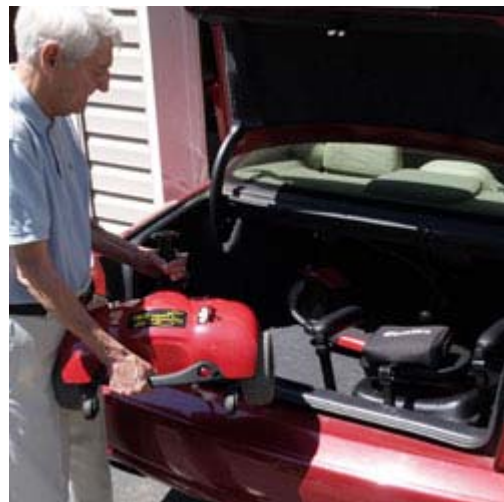
Figure 3: The Buzzaround 4-Wheel Scooter, model GB-104, from Golden Technologies, Inc. is a lightweight, portable scooter designed for indoor or outdoor use. It can be folded and broken down into components for easy storage or transport.
