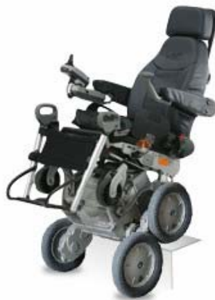
Figure 7: The IBOT from Independence Technology has wheels that rise or lower to aid in climbing stairs.
