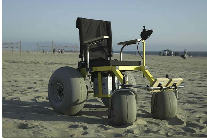
Figure 6: The Beach Cruzr from Hotshot Products is a powered beach chair with balloon wheels for moving on sand.
