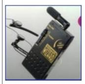
to face the person who is speaking (i.e. in a car). The units are pocket-sized and can be used with earphones, headphones, and neckloops. Some personal amplification systems have the option of adding modules that can be used in other listening environments as receivers for FM, infrared, or loop transmissions. A hardwired remote microphone at-
