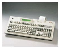
The Positron Express (left) functions as a TDD or TT machine when connected to a telephone and as an IBM compatible computer keyboard when connected to a PC. It also has a 4,000 character buffer that can be used to dump text from the
